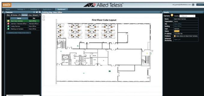
Auger building map has the exact location and state of the devices.
