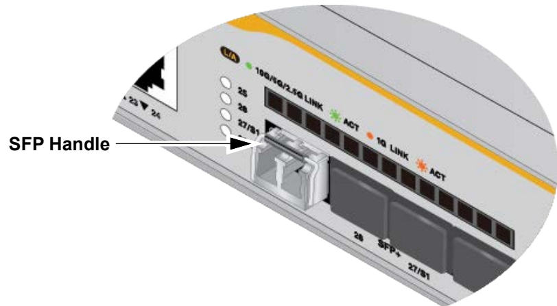
Figure 73. Positioning the SFP or SFP+ Handle in the Upright Position
