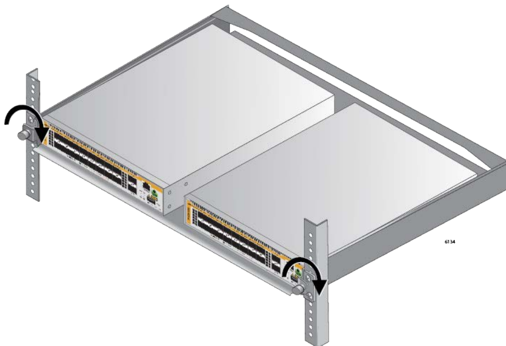
Figure 56. Tightening the Thumbscrews on the RKMT-J15 Rack Mount
