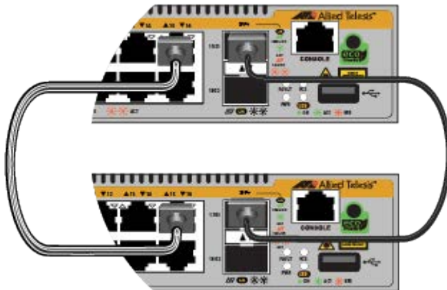
Figure 20. Stack Example with A Combination of Copper and SFP Ports
