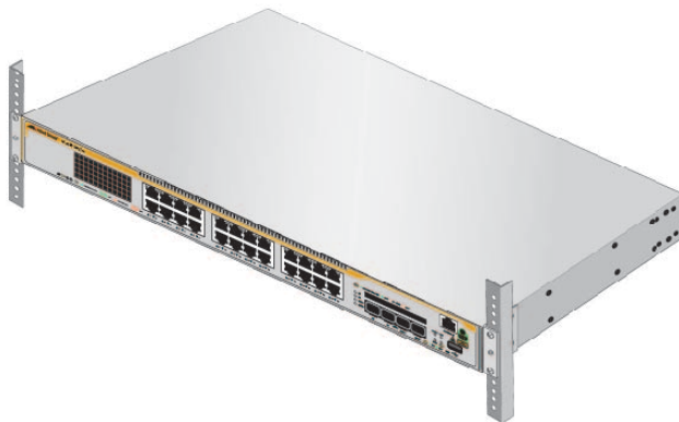
Figure 57. Correct Switch Orientation in an Equipment Rack
