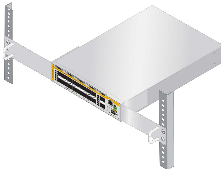
Figure 48. Installing the Switch in a Rack with the RKMT-J14 Brackets
