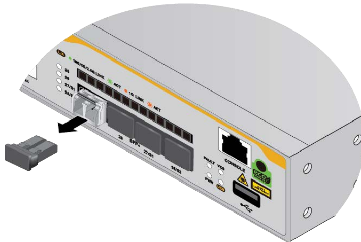
Figure 45. Removing the Dust Cover from an SFP or SFP+ Transceiver
