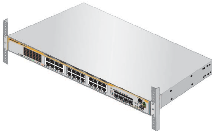
Figure 16. Correct Switch Orientation in an Equipment Rack
