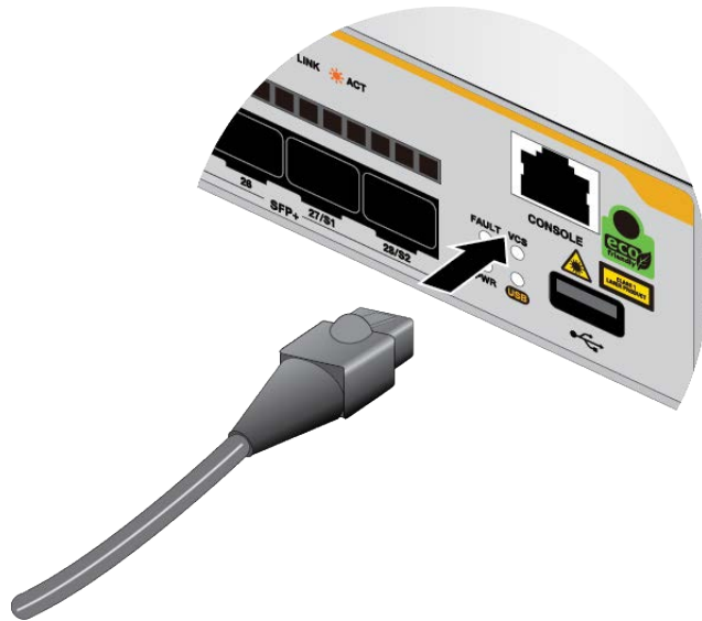
Figure 40. Connecting the Management Cable to the Console RS-232 Port
