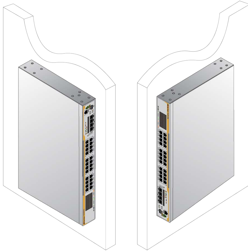
Figure 21. Correct Orientations of the Switch on the Wall
