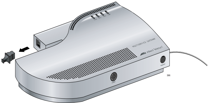
Figure 20. Removing the Plug from the Fiber Optic Port
